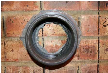
er 14/1/10 file: flood resistance test set-up
